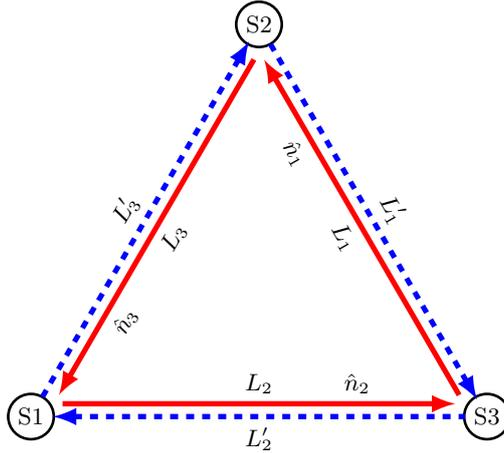
FIG. 8: Illustration of detector constellation. Three satellites are marked as 1, 2, and 3. Laser paths are marked as  $L_i$  and  $L'_i$ , where  $L'_i$  represents the direction opposite to  $L_i$ . The direction of unit vector  $\hat{n}_i$  is the same as that of  $L_i$ .
