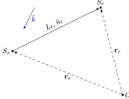
FIG. 7: A radio signal send from the point  $S_s$  travels along the arm  $L_l$  in the direction of  $\hat{\mathbf{n}}_l$  towards the receiver at  $S_r$ . The coordinate origin is denoted by  $O$ , while point  $S_s$  and point  $S_r$  are located at  $\mathbf{r}_s$  and  $S_r$ , respectively.
