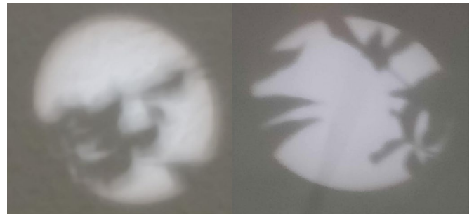
Fig 5a: Solar projections with obscurations. Left: Out of focus leaves close to the disco ball. Right: In-focus leaves situated further away from the disco ball.
