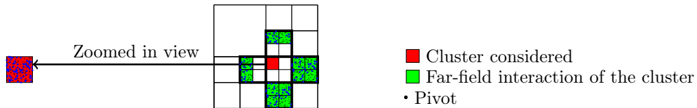
FIG. 10. Illustration of search spaces of the pivots in B2T NCA for nHODLRdD construction. Note that we consider only the far-field interaction here, i.e., \mathcal{IL}_{far}(X) \subset \mathcal{IL}_{HODLRdD}(X) .
