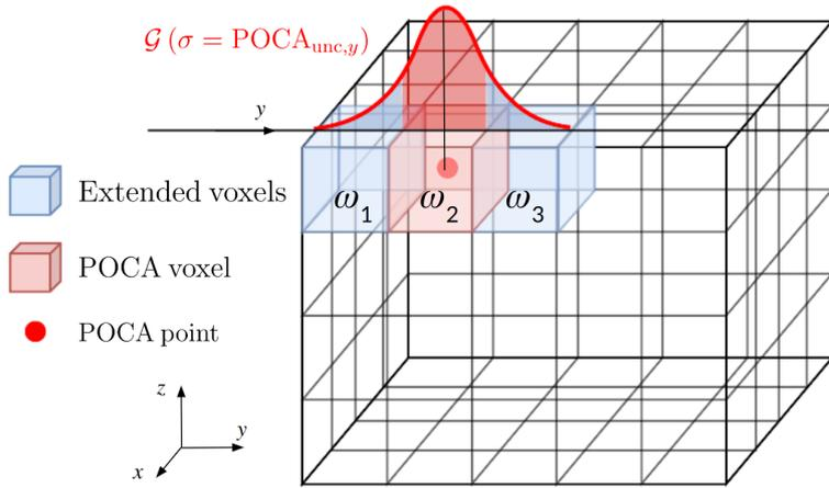
Figure 4: Illustration of PoCA point being extended to other neighbouring voxels with a Gaussian model. For the sake of readability, only the extension along the  $y$  dimension is showed.
