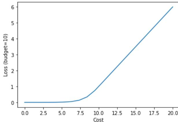
Figure 5: Example of the cost component of the loss as a function of detector cost, for a target budget of 10 A.U.. A sigmoid component below the budget provides a slowly increasing gradient as the cost approaches the target budget, beyond which the loss increases linearly. The function is fully differentiable.
