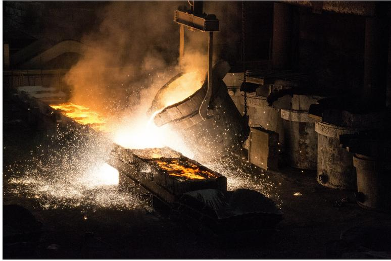
Figure 8: Example of a furnace ladle used in foundry industry. Image by Boris Bukovský, via Pixabay.
