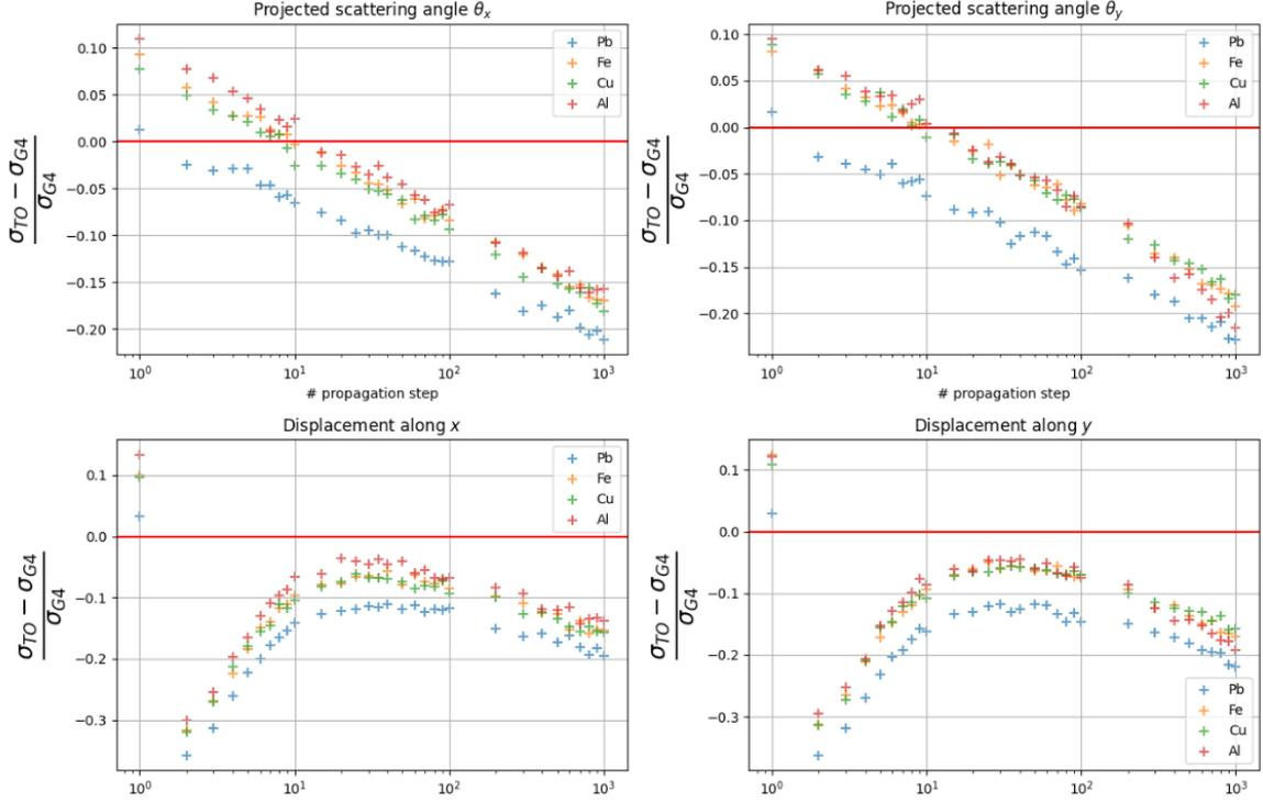
Figure 7: Comparison of standard deviations of projected scattering angles and displacement distributions between TOMOPT and GEANT 4 and for various number of propagation steps.
