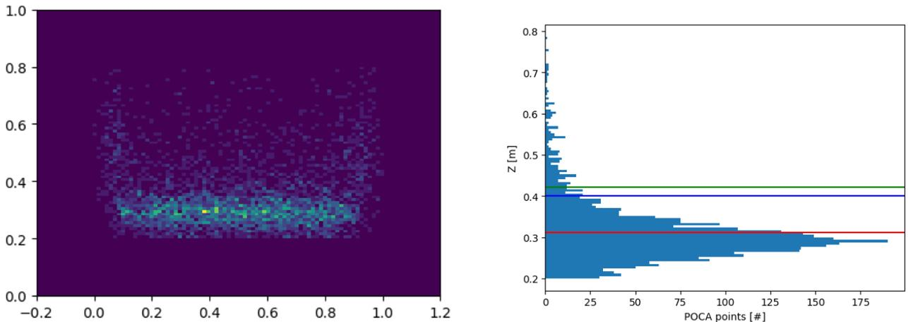
Figure 10: Muography of a simulation ladle furnace filled with steel up to 0.4 m. The bottom wall of the furnace goes from 0.2 m to 0.3 m in  $z$  axis. On the left, the front view of PoCA reconstruction. On the right, PoCA distribution in vertical axis ( $z$ ) and filling level inference example: true steel level (blue),  $\bar{z}_p$  (red), and  $h_{pred}$  (green) for the particular case of a bias correction on  $z_{pred}$ , with  $a = 2$  and  $b = -0.2$  (see Sec. 3.3.2 for details).
