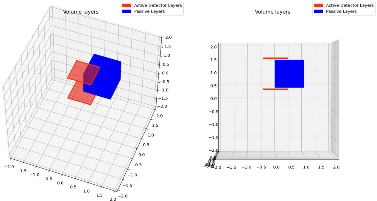
Figure 12: Initial layout of the detector panels above and below the passive volume.
