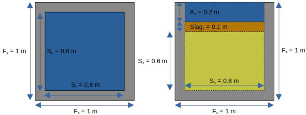
Figure 9: Top view (left), and front view (right) of the rectangular furnace ladle simulated. It is composed of walls (grey), liquid steel (yellow), slag (orange) and the air volume (blue) over the liquid steel and slag.
