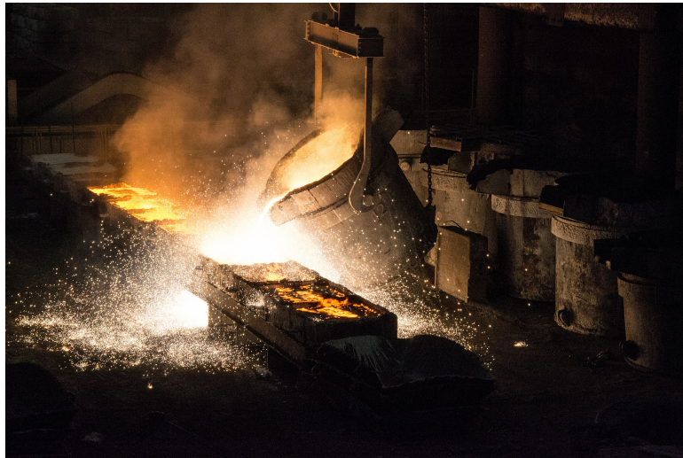
Figure 9: Example of a furnace ladle used in foundry industry. Image by Boris Bukovský, via Pixabay.
