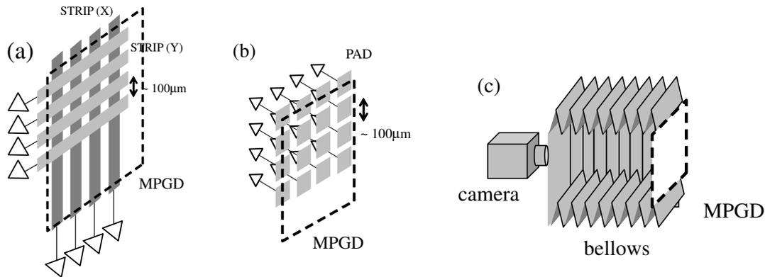
**FIGURE 5:** Schematic drawings of readout systems for gaseous TPCs. Panel (a), (b), and (c) show the strip charge readout, the pixel charge readout, and the optical readout, respectively.
