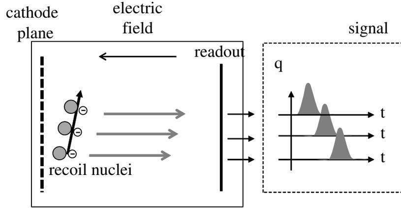
**FIGURE 3:** Conceptual drawings of a TPC. Ionization electrons or ions drift to the readout, and the differences in the drift length are projected on the time differences. For a more detailed explanation of the readout schemes, please see FIGURE 5.
