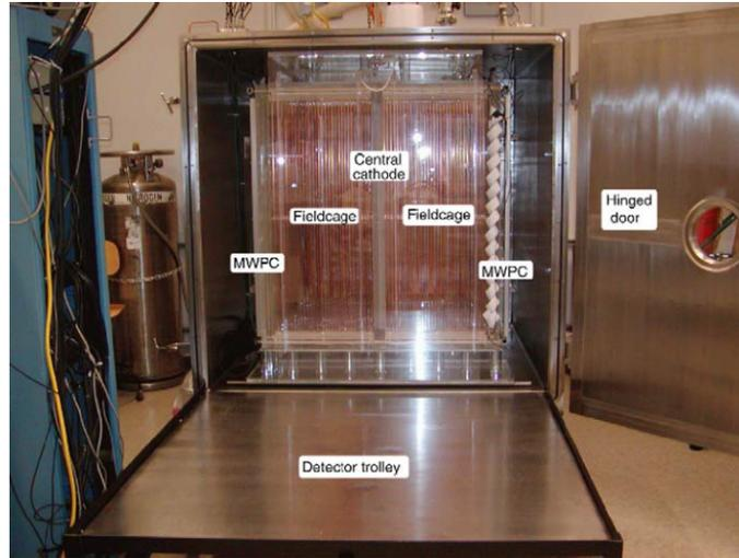
**FIGURE 4:** A picture of DRIFT-II, the first  $\mathcal{O}(1 \text{ m}^3)$ -sized detector in the field [50]. The central cathode is viewed by MWPCs at both ends. Tubular copper rings are held by a rigid Plexiglass support structure, forming the TPC field cage. The detector is placed within a stainless vessel.
