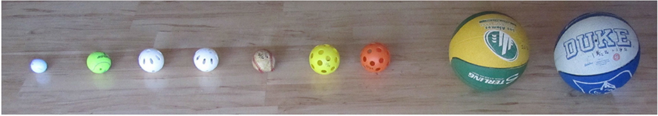
Figure 7. The experimental balls dropped from the bridge (de Silva et al., 2020). From left to right: golf ball, tennis ball, whiffle ball 1, whiffle ball 2, baseball, yellow whiffle ball, orange whiffle ball, green basketball, and blue basketball. Volleyball is not shown here.
