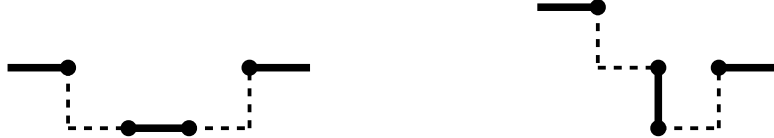
Figure 8: Sections of paths where we only keep one edge between two removed double-edges (dashed edges). The removed double-edges are non non-parallel resulting in non-minimal paths.
