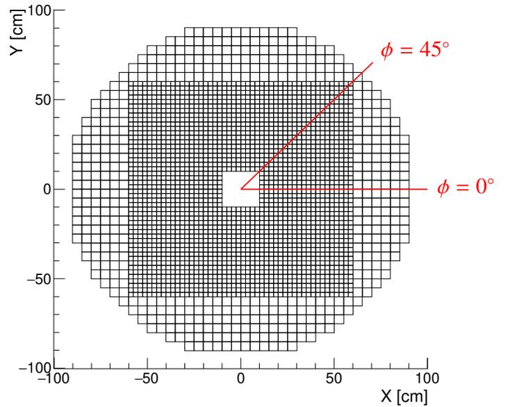
Figure 2: Eight-fold symmetrical layout of the CSI calorimeter viewed from downstream; this allows to mirror and fold a cluster at any location on the CSI surface to an equivalent location within the angular region of  $0^\circ \leq \phi \leq 45^\circ$ .
