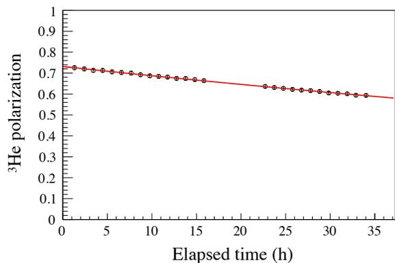
FIG. 5.  $^3\text{He}$  polarization versus elapsed time from the beginning of the measurement. The curved line shows the fit result by an exponential function. The measurement was not conducted from 16 h to 22 h due to a liquid He transfer for the superconducting magnet.
