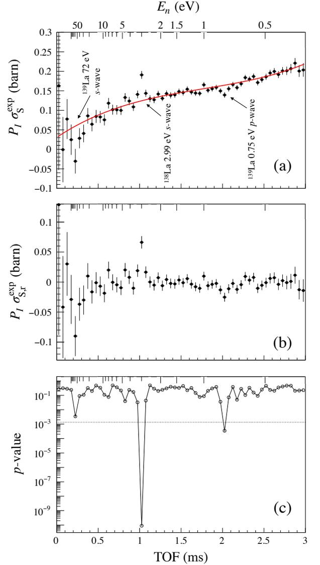
FIG. 7. (a) TOF dependence of  $P_I \sigma_S^{\text{exp}}$ . The curved line is the best fit of the global structure derived from the negative  $s$ -wave resonance. (b) Resonance component of spin-dependent cross section. (c)  $p$ -value for  $P_I \sigma_{S,r}^{\text{exp}}$ . The dotted line shows 99.7% confidence level.
