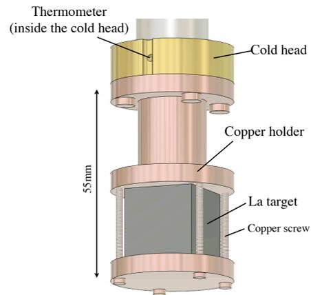
FIG. 2. Configuration around the La target. The thermometer was installed in the cold head.
