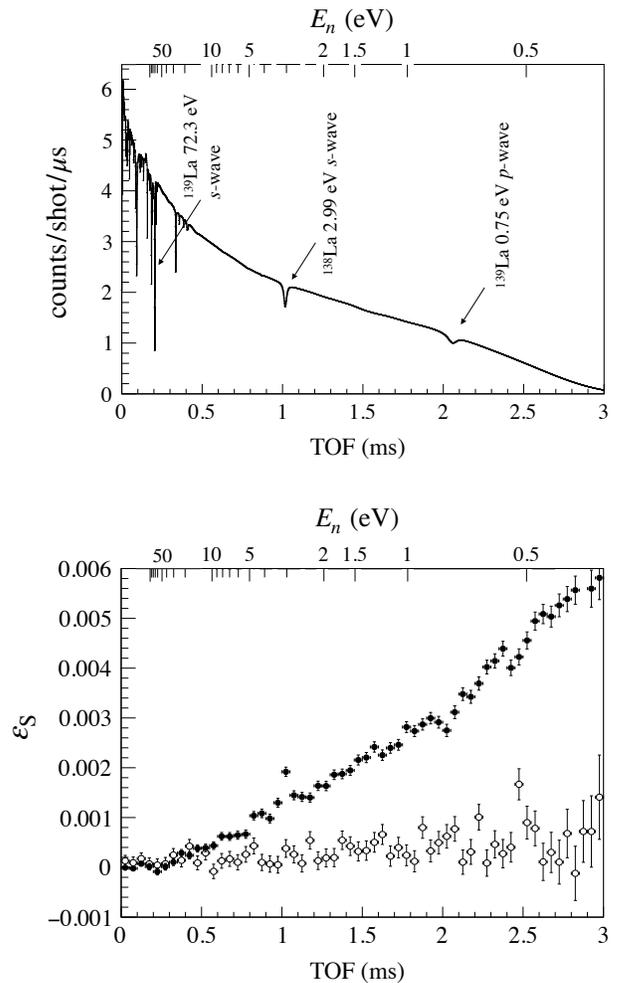
FIG. 3. TOF spectra of the transmitted neutrons (top figure) and the spin-dependent asymmetries (bottom figure). Black and white points denote the asymmetries in the conditions (a) and (b), respectively, in the bottom figure.
