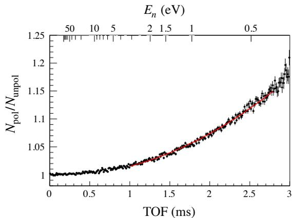
FIG. 4. Ratio of the counts of transmitted neutrons for the polarized to the unpolarized  $^3\text{He}$  spin filter. The curved line shows the best fit.
