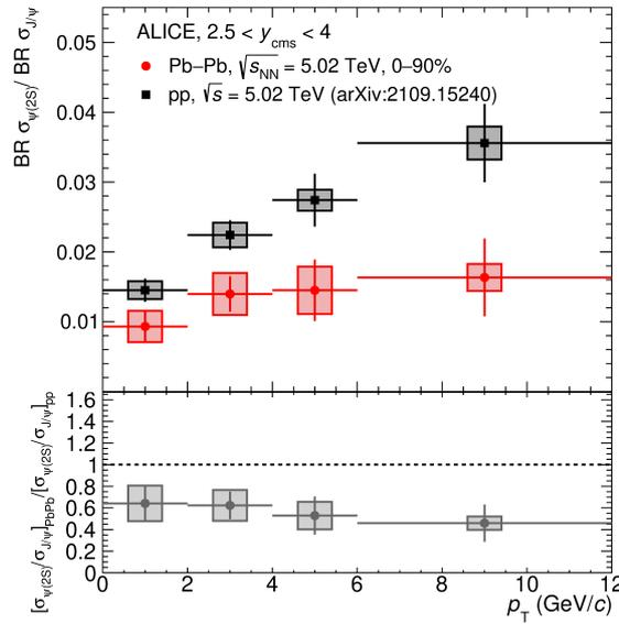
**Figure 4:** Ratio of the  $\psi(2S)$  and  $J/\psi$  cross sections multiplied with the dimuon branching ratios as a function of  $p_T$ , in Pb–Pb [1] and pp collisions [14]. In the lower panel the double ratio of the Pb–Pb and pp values is shown.
