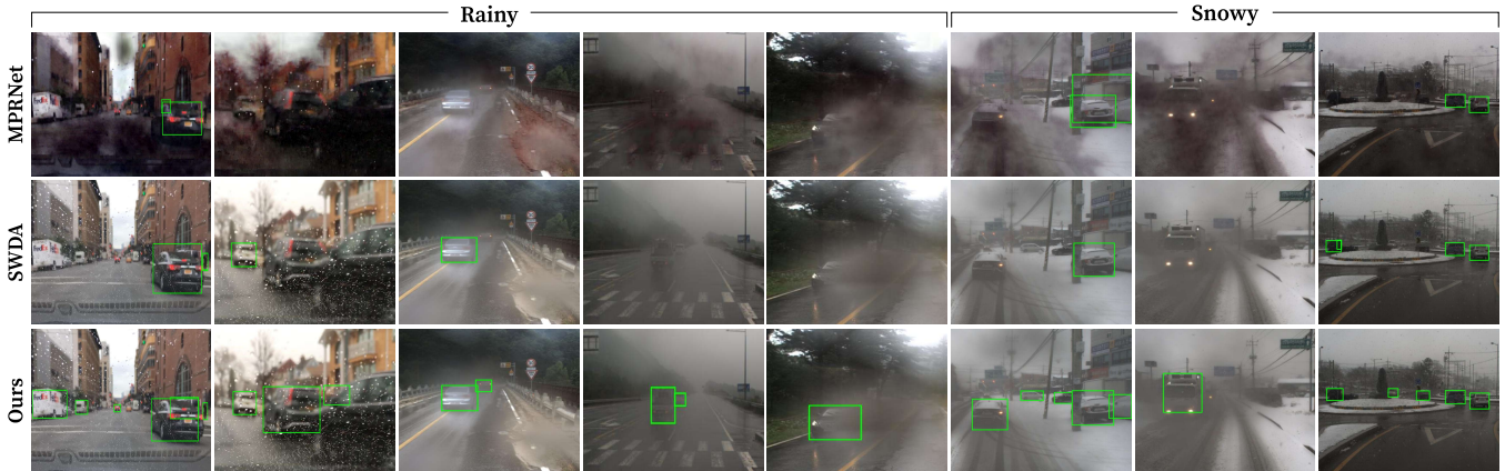
Fig. 3: Qualitative results on real-world target datasets. Compared to other methods, Ours successfully detects the objects even in the presence of severe weather corruption and style variations. Even though MPRNet removes raindrops in the first two images, the detector performance remains low, indicating images generated by the removal network do not consistently help object detection. In the remaining images, the removal network fails to remove corruptions and instead creates some artifacts due to the disparity between real weather data and synthetic weather data, which MPRNet was trained on. While SWDA directly adapts the network to the target domain, it fails to detect objects under severe weather corruption and environmental differences. More qualitative results are available in our multimedia material. [link]
