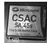
Figure 12: Space-rated radiation-hardened chip-scale atomic clock. Credit: Microsemi Product Catalog: https://microsemi.com/product-directory/embedded-clocks-frequency-references/5207-space-csac .
