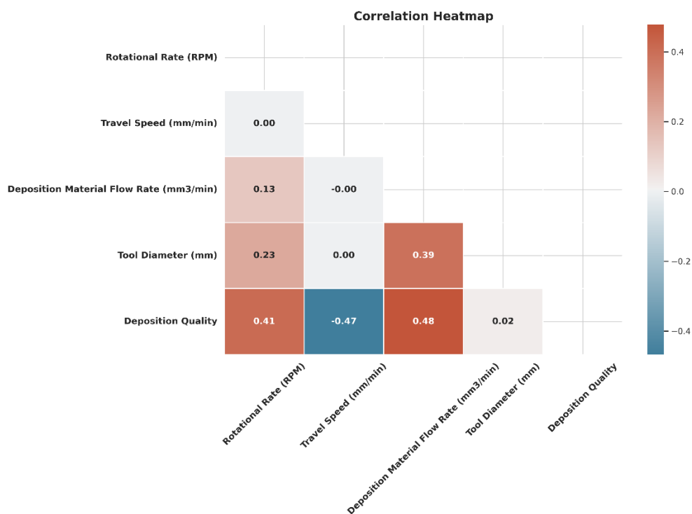
Figure 12. Correlation heatmap obtained to classify the deposition quality in the present work
