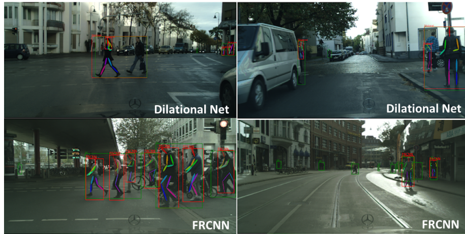
Fig. 24. On the top: Dilational Net can detect pedestrians even in the presence of occlusions, but produces one single bounding box for close by pedestrians. FRCNN can detect pedestrians that are close to the camera well, but fails to detect far away pedestrians.
