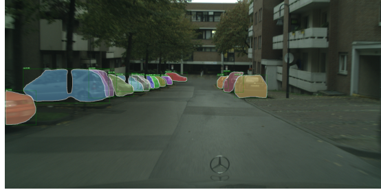
Fig. 19. PANNET correctly separates different parked cars even in the presence of occlusions.
