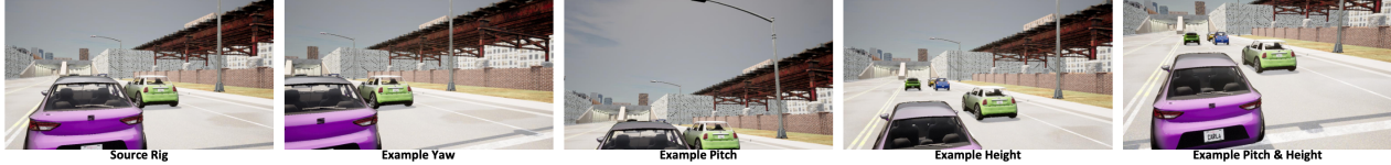
Figure 2. Datasets rendered in CARLA across viewpoints: For the analysis part of our work, we use CARLA to simulate different viewpoints. We rendered datasets from a total of 36 viewpoints, a few of which are highlighted above, including the source rig (extrinsics from nuScenes [2] dataset), +12^\circ yaw, +12^\circ pitch, +21 inch height, and -12^\circ pitch and +18 inch height together.
