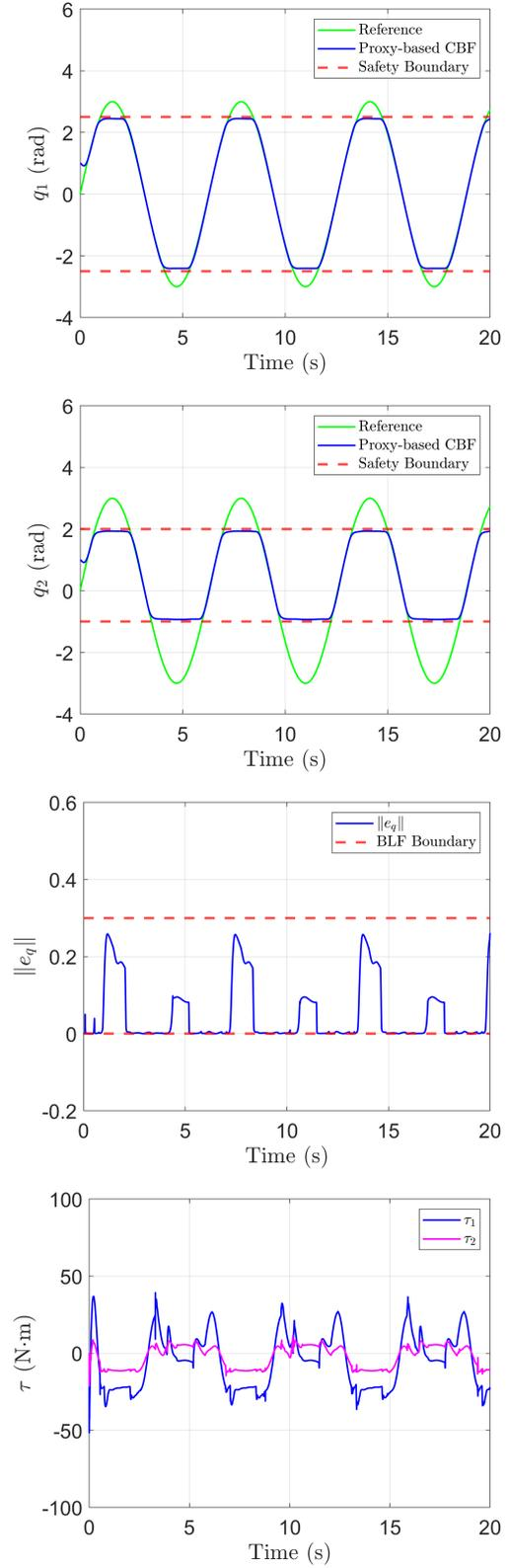
Fig. 2. Simulation results of the joint space safe control. From (a) and (b) it can be seen that the proposed controller can ensure safety of  $\mathcal{C}_q$  as the trajectories of  $q_1$  and  $q_2$  never cross the boundary of the safe region represented by the dash red lines, with good tracking performance inside the safe region. Moreover, from (c) one can conclude that the adaptive BLF-based controller developed in Theorem 1 is effective since the constraint on  $e_q$  is not violated.
