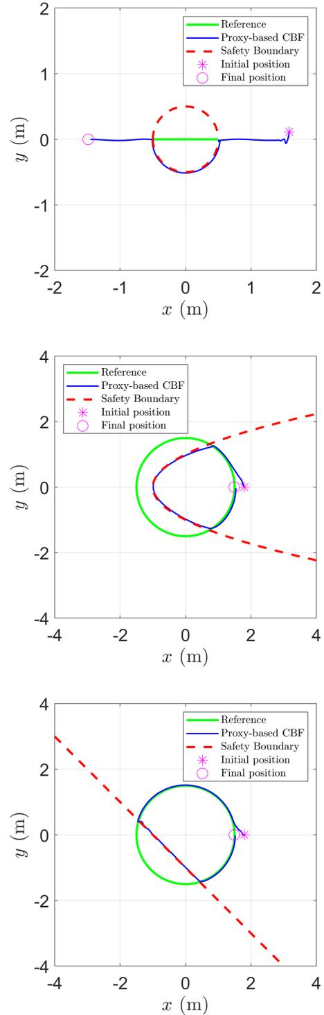
Fig. 3. Simulation results of the task space safe control. One can observe that proposed controller can ensure safety of  $\mathcal{C}_p$  as the trajectories of  $x$  and  $y$  always stay inside the safe region whose boundary is represented by the dash red lines, and the tracking performance inside the safe region is satisfactory.
