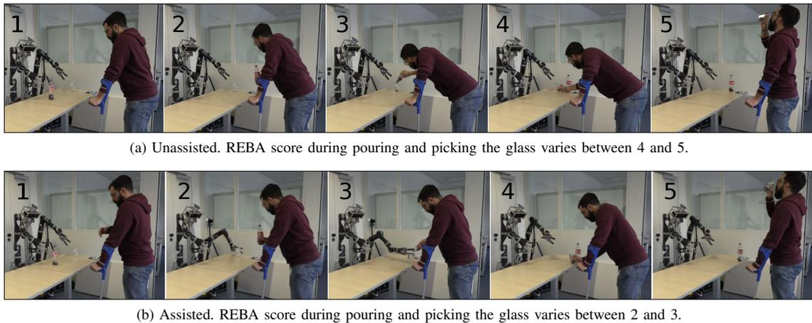
Fig. 9. Keyframes of the robot-assisted pour-bottle-into-glass task. By comparing keyframes 3 and 4 for the two cases, we can observe the effect that the robot interventions have in the human posture.
