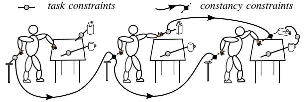
Fig. 3. Illustration of the constraints used to describe the first three keyframes of Fig. 2 with the robot and its actions being omitted for clarity. *Task constraints* are used only within keyframes and *constancy constraints* are used between keyframes, hence they are illustrated with arrows to link timeframes and diamonds to indicate which dimensions remain constant.
