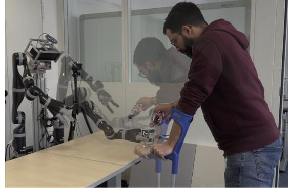
Fig. 1. Illustration of the presented concept in a supported pour-bottle-into-glass task. A robot intervenes to move the glass (transparent view) to a location on the table that enables an impaired user to comfortably pour the content of a bottle into it. The supported human (solid view) is enabled to perform the task optimally given an ergonomic metric. In the non-supported case, the (transparent) human needs to get into an uncomfortable posture.
