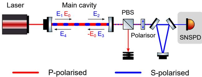
FIG. 1. **Schematic of the experimental setup.** P-polarised pump light resonates in a main linear optical cavity. The ALP field converts a small portion of light into S-polarised at a shifted frequency, which is isolated by a series of polarised optics and triangular optical cavities. The signal field is detected by a superconducting nanowire single photon detector (SNSPD). PBS: polarising beam splitter.
