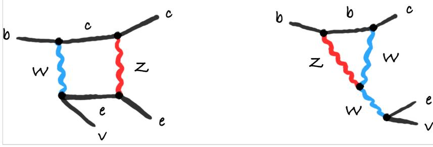
**Figure 8.** Examples of Feynman diagrams that contribute to the short-distance EW corrections encoded by the Wilson coefficient  $C(\mu)$ . Only contributions involving  $Z$ -boson exchange are shown but there are also photon loops.
