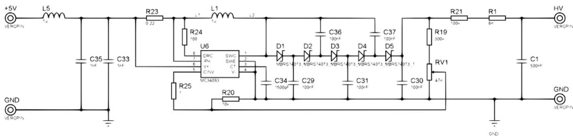
Figure 1. The high voltage converter circuit diagram.
