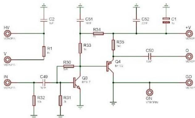
Figure 2. The circuit diagram of the preamplifier.
