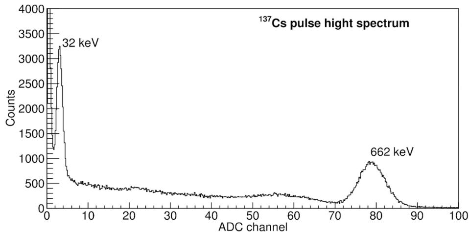
Figure 6.  $^{137}\text{Cs}$  spectra on count and energy mode.
