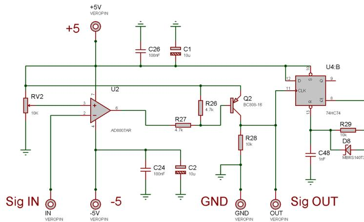
Figure 3. The circuit diagram of the comparator.
