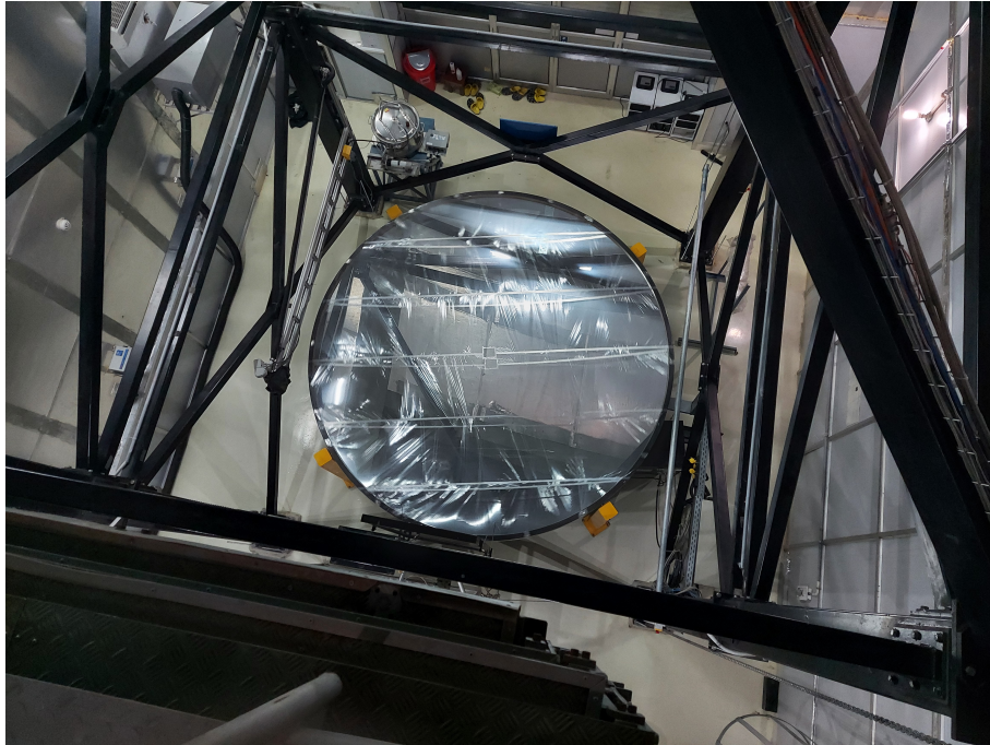
Figure 3: A top view of the ILMT showing the liquid mercury mirror covered by a mylar film.
