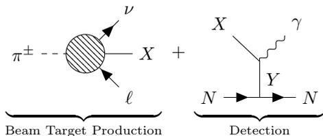
This simple setup was shown to explain the MiniBooNE excess in ref. [44], making use of two prominent features; (I) the coupling of a boson  $X$  to the charged pion decays
