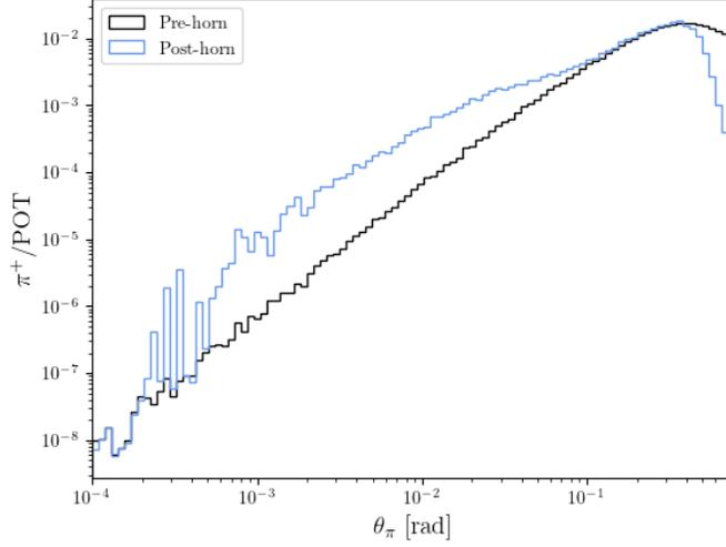
FIG. 12. The pre-horn  $\pi^+$  flux (black) using the Sanford-Wang parameterized cross section convolved with the BNB proton beamspot, and the post-horn flux (blue) after modeling the transport through the magnetic horn system are both shown as a function of the pion angle with respect to the beam axis. In both cases  $5 \cdot 10^5$  simulated POT were used.
