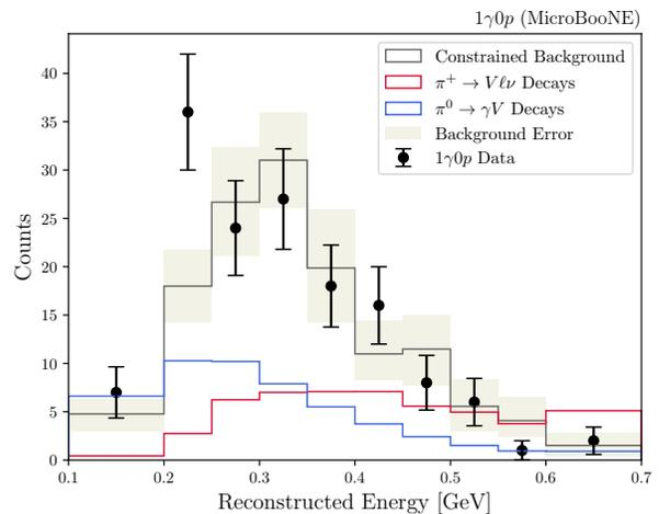
FIG. 5. Example event spectra prediction from 2-body decays of  $\pi^0 \rightarrow \gamma V$  (blue) and 3-body decays of  $\pi^+ \rightarrow \ell \nu V$  (red) at MicroBooNE in the  $1\gamma 0p$  topology. Here the LLP mass  $m_V$  is fixed to 5 MeV.
