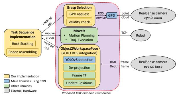
Fig. 2. Generic software architecture based on vision-based frameworks.
