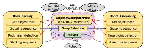
Fig. 5. Rock stacking and Assembly tasks vision-based frameworks.
