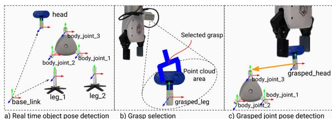
Fig. 7. Main steps for the robot assembly task.
