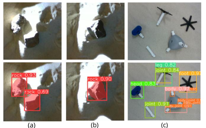
Fig. 4. Custom datasets and YOLOv8 predictions (a) moonrock segmentation (b) moonrock segmentation, mask deformed by strong exposure (c) robot components detection.
