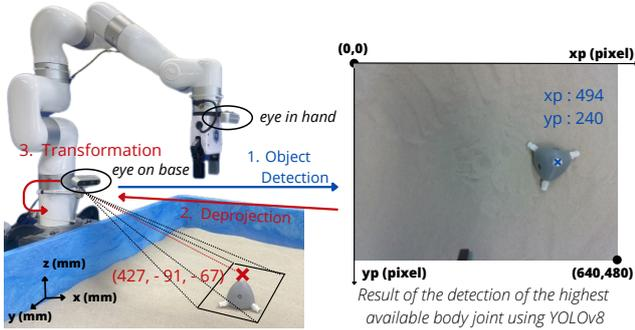
Fig. 6. Scheme of the *pixel to point* process.
