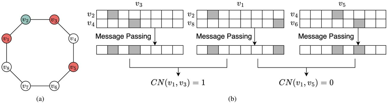
Figure 1: (a) Isomorphic nodes result in identical MPNN node representation, making it impossible to distinguish links such as  $(v_1, v_3)$  and  $(v_1, v_5)$  based on these representations. (b) MPNN counts Common Neighbor through the inner product of neighboring nodes’ one-hot representation.
