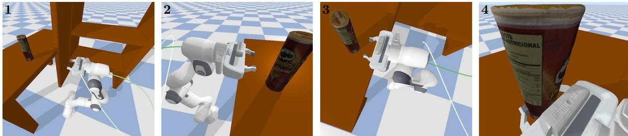
Figure 2: A sampled trajectory for grasping a can. Frames 1-2, 2-3, 3-4 depict respectively the end-effector alignment with the final pose, the approach stage, and the grasping stage.
