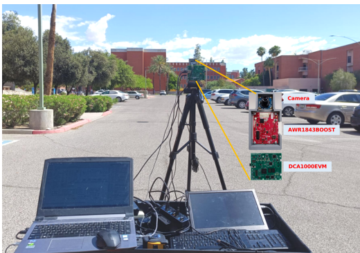
Fig. 5: The experimental setup, where a laptop and an NVIDIA Jetson Xavier GPU establish a connection with the radar-camera system using Ethernet and USB cables to collect data.
