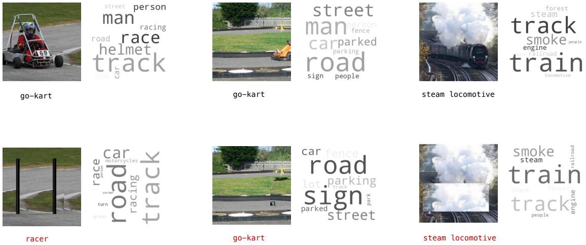
Figure 2: Class predictions and corresponding word clouds generated by TExplain for both the original (top) and Only-BG-T (bottom) samples extracted from the Background Challenge dataset. The class predictions are displayed below each image.
