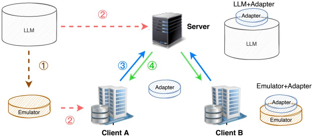
Figure 2: The unified interfaces for federated fine-tuning LLMs with or without accessing the full model. When the LLM is not accessible to clients, different algorithms can be used to generate an emulator, including distillation, pruning, and quantization via ① LLM model pre-processing interface; if the LLM is accessible, ① just output the input by default. The other three interfaces in the figure are ② initial model broadcast, ③ shared parameter aggregation, and ④ parameter re-distribution.
