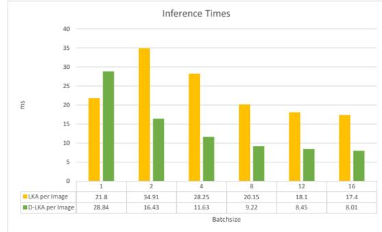
Figure 7. The inferences time in ms for an input image of size  $3 \times 224 \times 224$  on the 2D methods. The times are already calculated for a single image for better comparison.
