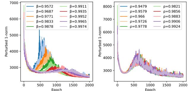
Figure 6. Plots of  $\|\nabla E\|_{1,\varepsilon}$  after each epoch for full-batch Adam,  $h = 10^{-4}$ ,  $\varepsilon = 10^{-8}$ . Resnet-50 on CIFAR-10, left:  $\rho = 0.999$ , right:  $\beta = 0.97$ .
