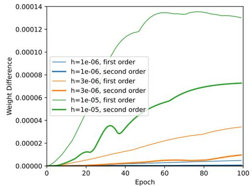
Figure 3.  $\|\theta^{(n)} - \tilde{\theta}(t_n)\|_\infty$  for a MLP trained with full-batch Adam on truncated MNIST, where  $\tilde{\theta}(t_n)$  is either first (signGD perturbed by  $\varepsilon$ ) or second order approximation to Adam;  $\beta = 0.9$ ,  $\rho = 0.95$ ,  $\varepsilon = 10^{-6}$ . Precise definitions are provided in Appendix H, specifically (63).
