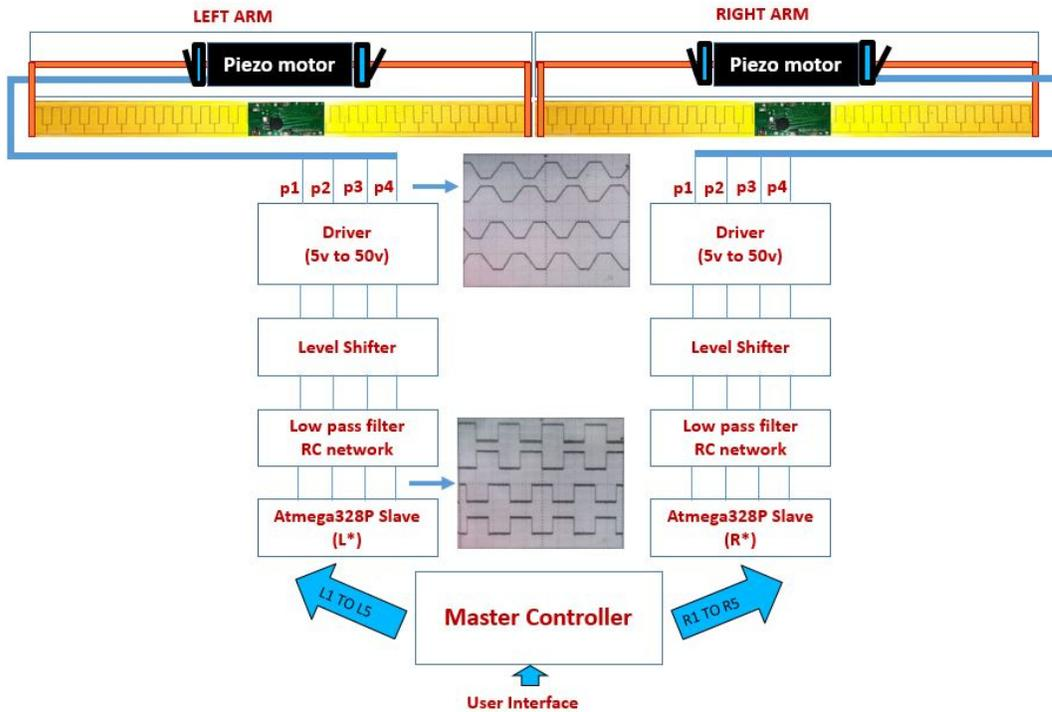
Fig. 3. Schematic to show the working principle of the functional blocks of the controller electronics for the piezowalkers.
