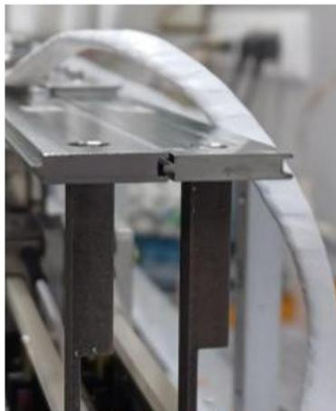
Fig. 2. Cross-section of the single slit bar designed to allow smooth motion without light leak. The copper braids used to cool the slit bars are also shown.
