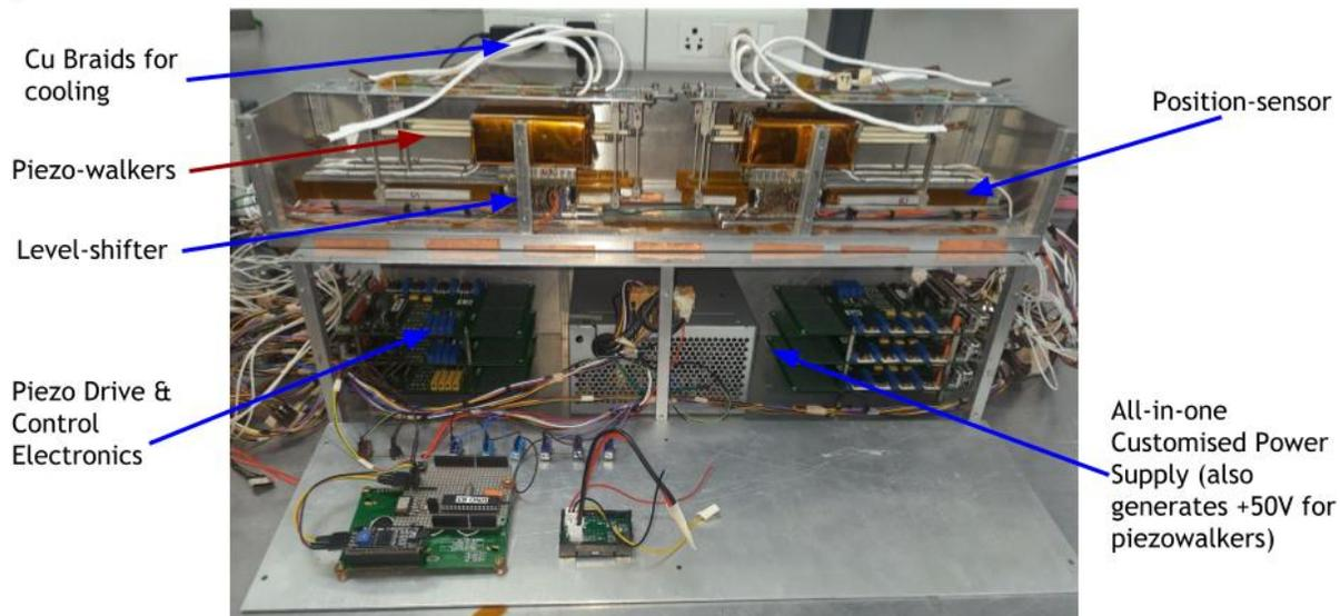
Fig. 4. Completed CSU prototype creating 3-slits at the FOV in the laboratory. The slit bar assembly on the top will be inside the cryogenic dewar while the drive and monitoring electronics will be outside.
