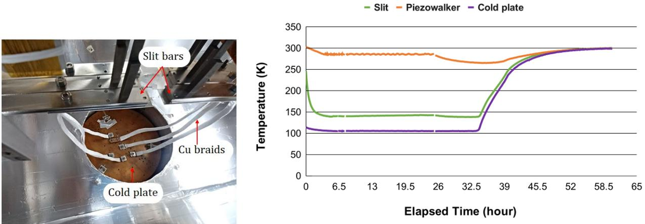
Fig. 5. (Left) The CSU connected to the cold plate (at the bottom of the liquid  $N_2$  tank) inside the dewar prior to the cryogenic testing of the unit in the laboratory. The shinning surface around the cold plate is a radiation shield created to ensure efficient cooling by reflecting the heat due to the uncooled parts of the dewar. (Right) Typical temperature profiles of the slit bar, the body of the piezo-walker and the coldplate measured during one of the cryogenic tests in the laboratory.
