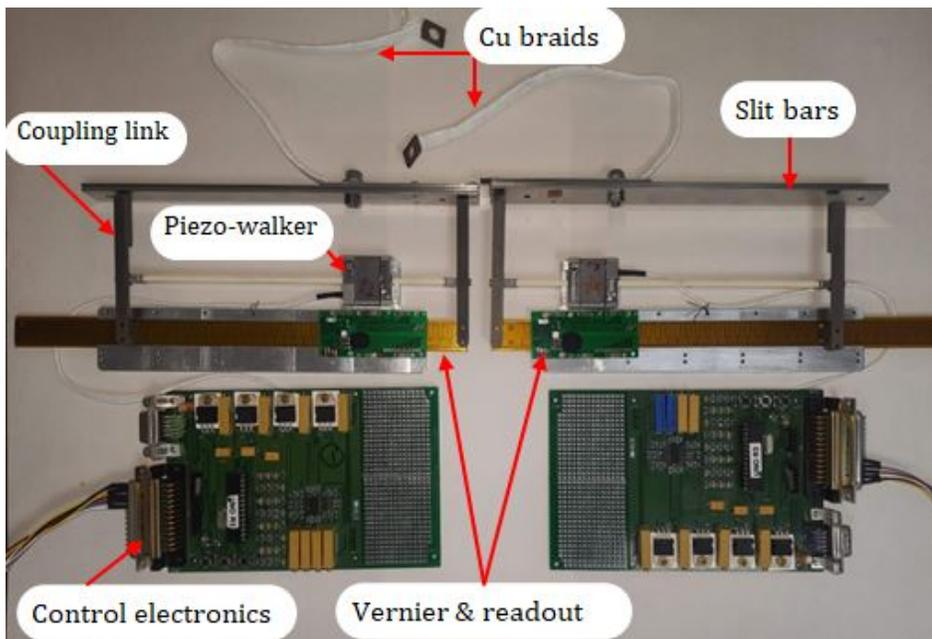
Fig. 1. Single slit pair assembly along with the drive electronics. The functional components of the bar assembly are labeled.
