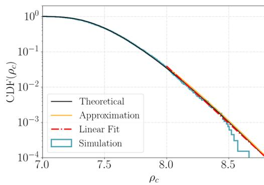
FIG. 10. Cumulative density distributions obtained by integrating Eqs. A10 (black) and A12 (orange), along with a histogram (blue) from simulated results. A linear fit (red) is overlaid in the logarithmic scale for comparison.
