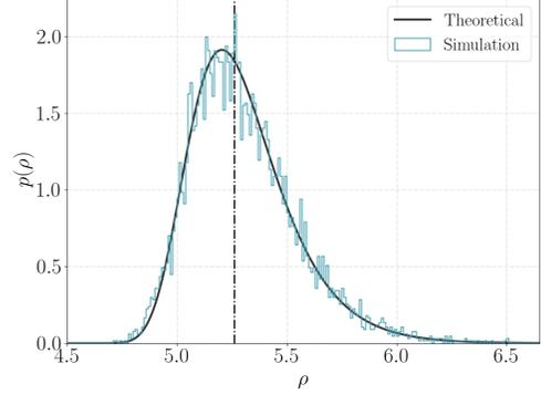
FIG. 8. Probability density function of  $\rho$  represented as a histogram (in blue). An ideal Rayleigh distribution is overlaid in black, providing a visual comparison. The vertical dotted line represents  $\rho = 5.3$ .
