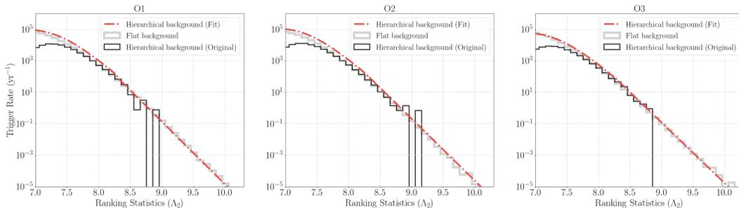
FIG. 5. Comparison of the histograms of background trigger rates (excluding the foreground) versus ranking statistics for O1, O2, and O3 data. The black curve represents the true background obtained from time-shifted triggers across the detectors. The red curve represents the background obtained after fitting the true background trigger distribution. The background trigger rate from a flat search is overlaid in gray for comparison.
