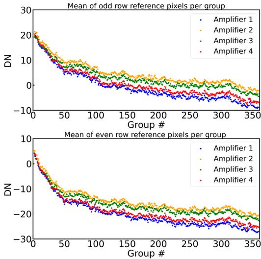
**Figure 15.** The average of the even and odd reference pixels for each amplifier from a dark exposure with 360 groups. This mean is made after the first group was subtracted. The mean reference pixel for group 1 for all the cases is zero. Over-plotting of the amplifier points obscures this mean of zero for amplifiers 2-4
