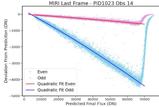
**Figure 6.** A plot showing the systematic offset in the last group of each integration from the predicted flux based on the prior count rate. Odd rows show an offset of approximately 6%, while even rows show an offset of only about 1%. The trendlines are given by a second degree polynomial to account for the slight non-linear shape of the effect, but are dominated by the linear term. As the final group approaches saturation, the effect goes away.
