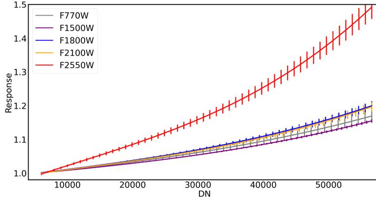
**Figure 7.** Response curves and uncertainties for Imager detector. Here the response, y-axis, is the ratio of the a linear fit to the pixel ramps/ raw DN values of the pixel ramps. The wavelength-dependence of the non-linearity correction is evident from the divergence between the F1500W and the F2500W response curves.
