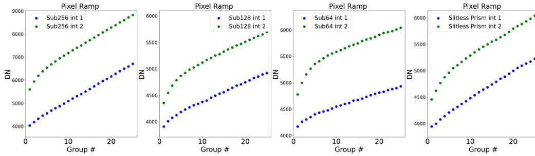
**Figure 10.** The RSCD effects are illustrated for subarray exposures with two integrations. The blue points are the first 25 groups of the pixel ramp for the first integration, while the green points are the same pixel ramp for the second integration. The plots from left to right are pixel ramps for the SUB256, SUB128, SUB64, and SLITLESSPRISM subarrays
