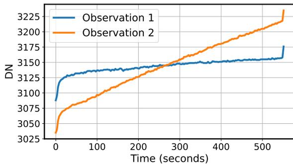
**Figure 13.** Median MRS ramps in a roughly 6000-pixel dark region in the middle of the short-wavelength detector. Observation 1 (orange line) and Observation 2 (blue line) are identically-configured observations taken two days apart, targeting shielded areas within already nearly-empty fields and shows dramatically different effective dark count rates.
