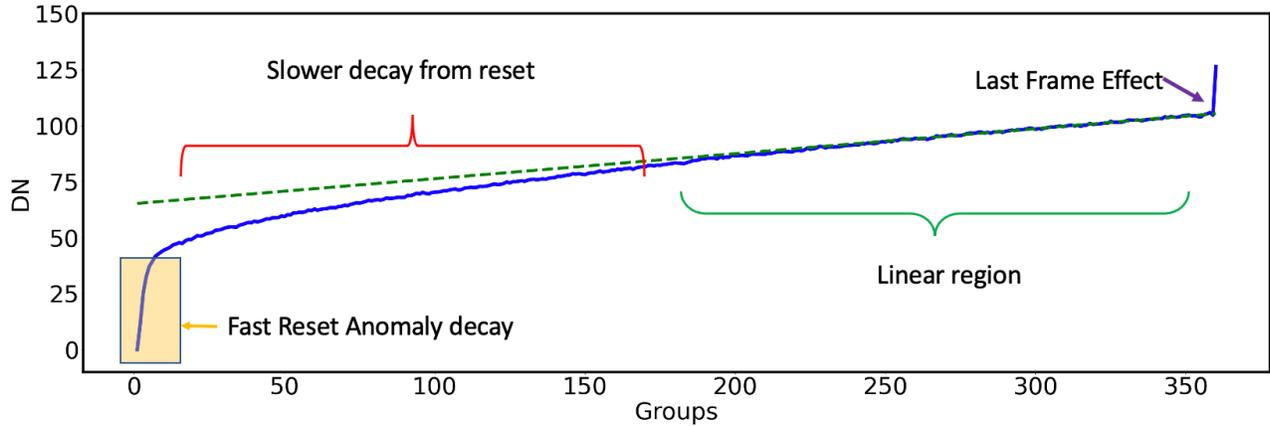
**Figure 12.** Plot of a long dark exposure. The first group has been subtracted from each pixel ramp so that each ramp starts at 0. The blue line is the median of all the pixels at each group after sigma clipping for outliers caused by hot pixels, dead pixels and cosmic ray effects. The accumulated signal is not linear with time. The dashed green line is a linear fit to the last 150 groups.
