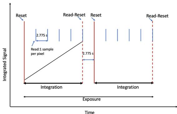
**Figure 3.** The sampling up-the-ramp for the FASTR1 mode read-out scheme for a single pixel. In this example  $N_{\text{sample}} = 1$ ,  $N_{\text{groups}} = 5$ , and  $N_{\text{int}} = 2$ . The x-axis is time and the y-axis is signal strength. Each blue vertical tick marks a read of the pixel and each red vertical tick marks a reset of the pixel. In this scheme, each reading of a pixel will have only one sample at each pixel. The time to read an entire group is 2.775 s.
