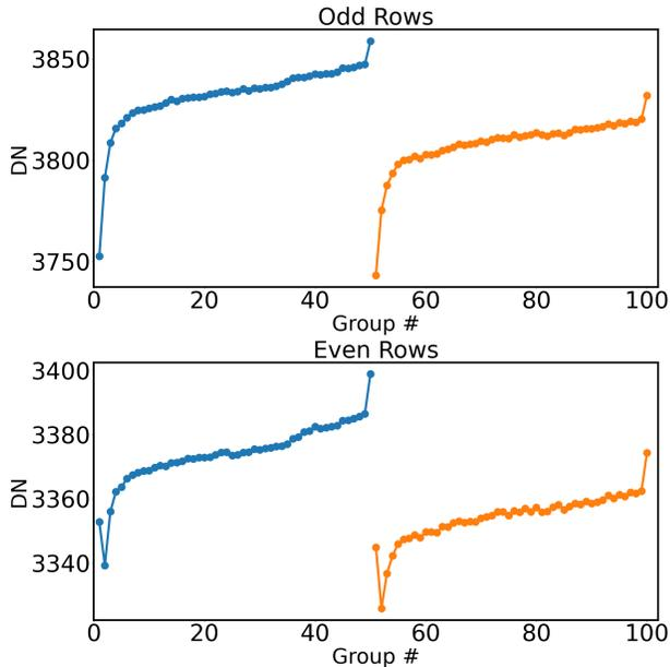
**Figure 11.** Top: Mean ramp of neighboring odd pixels for the first (blue points) and second (orange points) integration. Bottom: Mean ramp of neighboring even pixels for the first and second integration. 200 pixel ramps were averaged to make the mean ramp, with sigma clipping to remove the effects of cosmic rays.
