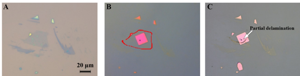
Fig. S13 Optical characterization of a failed exfoliated graphene device. (A) Optical
