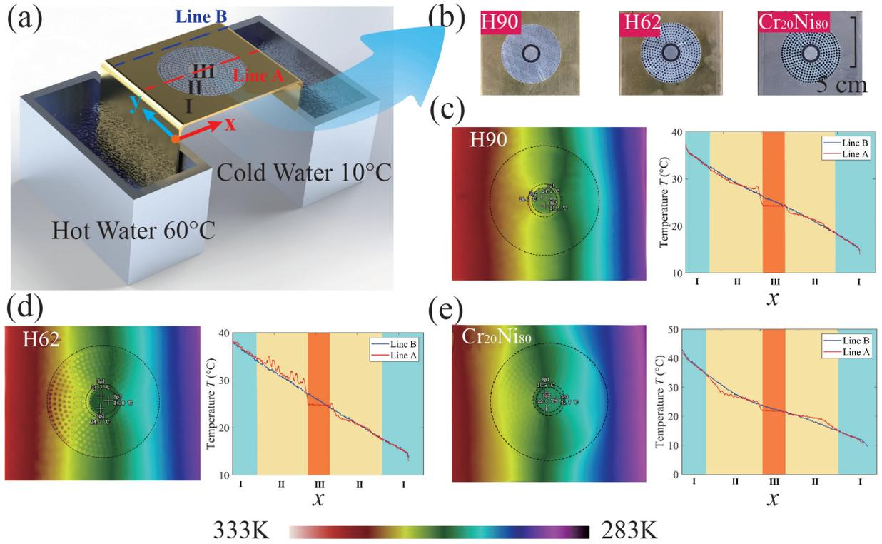
FIG. 4: Experimental devices and demonstrations. (a): The experimental device. The left tanker is filled with hot water at 60 °C and the right at 10 °C. (b): Three specimens with different backgrounds. The experimental results are shown in (c), (d) and (e). The host block (background) is Brass H90 in (c), Brass H62 in (d), Cr<sub>20</sub>Ni<sub>80</sub> in (e).
