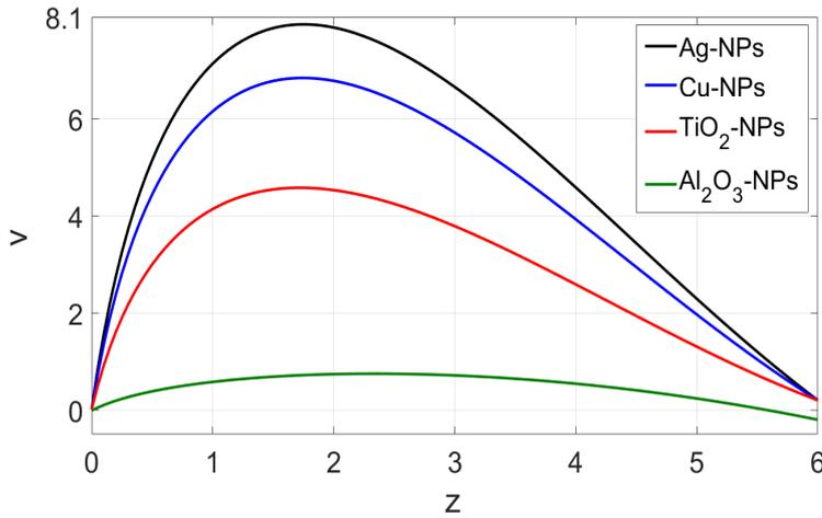
**Fig. 6** The influence of various NPs on axial velocity
