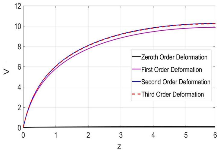
**Fig. 3** Convergence of HPM using various orders of deformation of axial velocity.
