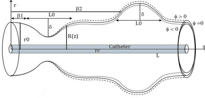
**Fig. 1** Schematic representation of a vascular model.
