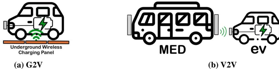
Figure 1 Different types of Dynamic Wireless Charging
