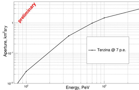
**Figure 5:** Expected Terzina aperture to protons' EAS vs energy during the first year of operation.
