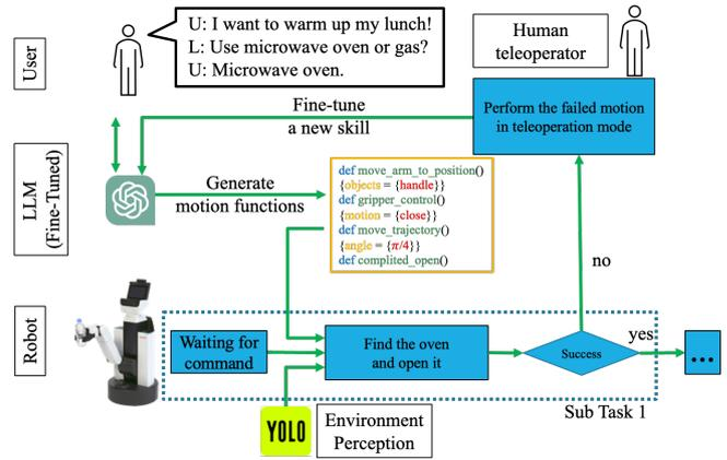
Fig. 1. Framework of LLM-based task planning with enhanced HRC.
