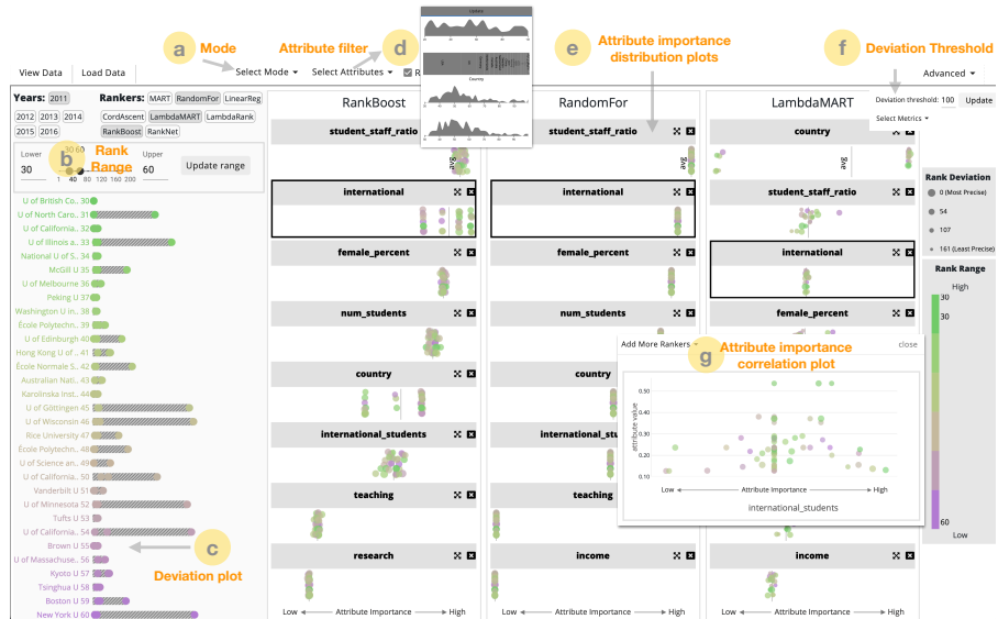
Fig. 3 Visualization Interface for TRIVEA: The control panel on the left comprises options to select: (a) different modes of comparison, such as Ranker mode, Range mode, and Time mode, (b) a group of items by rank range, (d) a group of items by attribute values, and (f) the permissible deviation threshold. The visualizations shown are: the deviation plot (c), which encodes the goodness of fit for the learned rankings; attribute importance distribution plots (e), which shows the attribute importance distribution (x-axis) among the items in the selected range, attribute importance correlation plots (g), which shows the attribute importance (x-axis) versus the ground truth value (y-axis). In (e), we add jittering along the y-axis to minimize overlapping. The Y-axis does not carry any meaning. The attributes are sorted from top to bottom according to the attribute average importance score for the given range and ranker.
