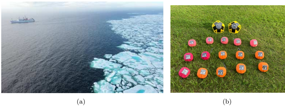
Figure 4. (a) Photograph taken by Tomotaka Katsuno showing the sea ice edge where wave buoys were deployed from R/V Mirai in MR22 cruise. (b) Wave buoys prepared for the MR22 cruise. Although only two Spotter buoys are shown in the photo, three Spotter buoys were deployed.
