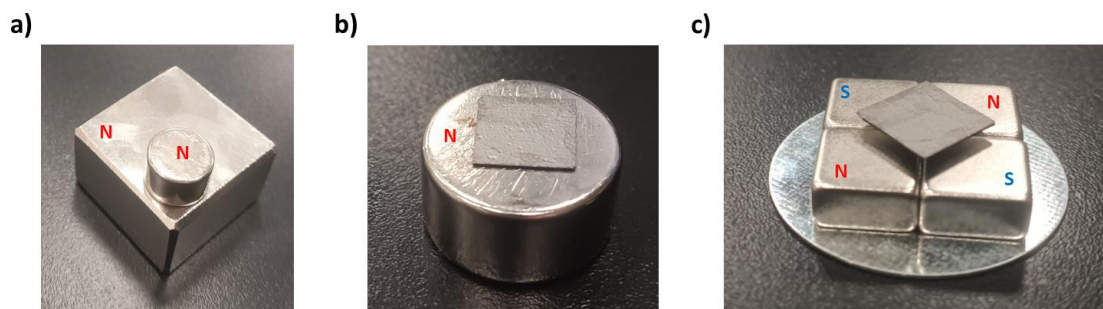
Figure 2. Experimental final resting place of a) A small cylinder magnet No.1 on a big cuboid magnet No.3. b) A piece of diamagnetic pyrolytic graphite touching the surface of a big cylinder magnet No.2. c) A piece of diamagnetic pyrolytic graphite levitated over a magnet array.
