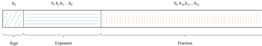
Fig. 2. The sign field in IEEE 754 floating-point numbers determines the sign of the floating-point number, the exponent field determines the position of the decimal point, and the fraction field determines the significant digits.
