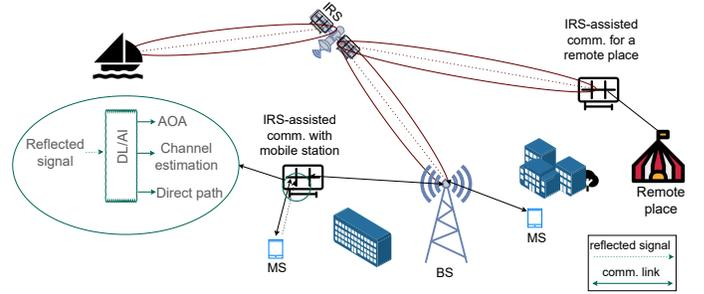
Fig. 8. Schematic representation of an IRS-assisted ISAC system.
