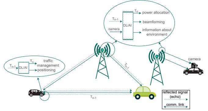
Fig. 6. An illustration of a vehicular network that utilizes ISAC where: 1) A BS communicates with vehicles and uses the reflected signal for sensing purposes. 2) Two vehicles communicate with each other and utilize the reflected signal for traffic management.
