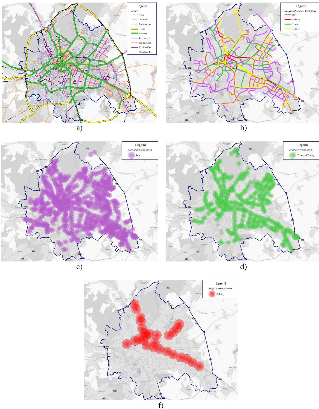
Fig. 4. Basic characteristics of the transport system of Kharkiv, represented in PTV Visum model: a) road network; b) public transport network; c) spatial coverage of bus stops; d) spatial coverage of tram and trolleybus stops; e) spatial coverage of metro stations
