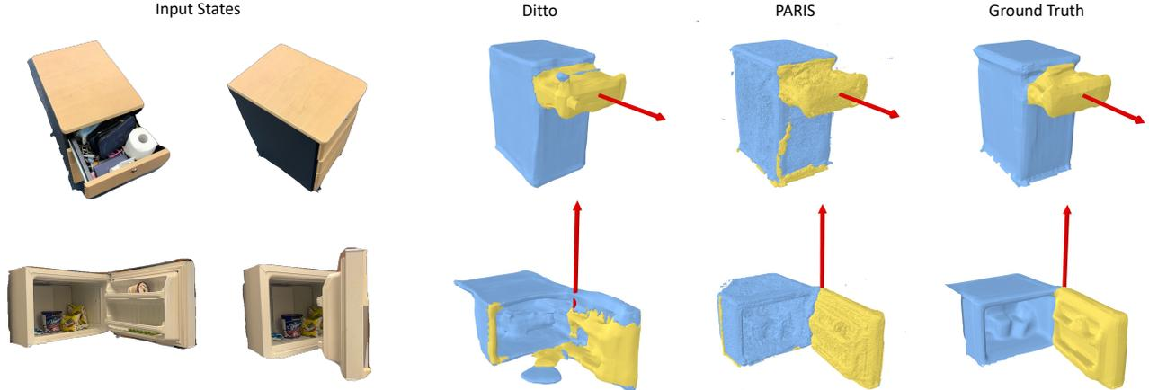
Figure 6. Qualitative results for two real-world objects. Ditto and our method can both estimate accurate motion parameters. Ditto produces cleaner segmentation in the first case, but a less accurate geometry in the second case.
