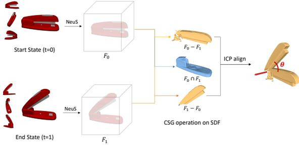
Figure 4. Pipeline of our baseline method *Ours-ICP*. We learn separate neural SDFs  $F_0, F_1$  for the object in state  $t = \{0, 1\}$ . To segment static and movable parts, we apply CSG operations between two SDFs. Then we leverage global registration and the ICP algorithm to obtain the transformation on the movable parts from the start to end state.
