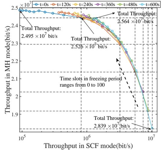
Fig. 16: The Tradeoff Between Throughput in SCF Mode and in MH Mode.
