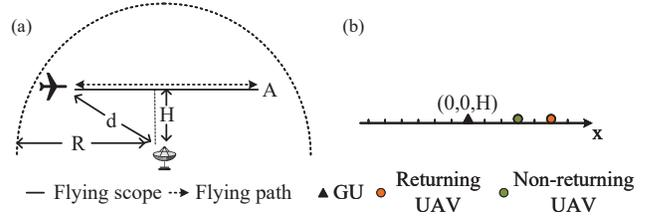
Fig. 5: UAVs' 1-D space of activities. (a) the scene diagram of the UAV's activity range in 1-D. (b) the top-view geometric diagram of the UAV's activity range in 1-D
