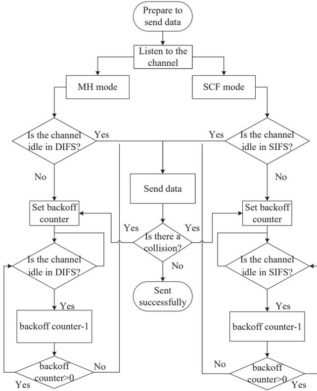
Fig. 3: Control channel access mechanism.
