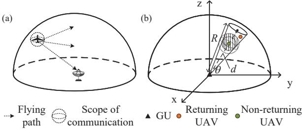
Fig. 7: UAVs' 3-D space of activities. (a) the scene diagram of the UAV's activity range in 3-D. (b) the geometric diagram of the UAV's activity range in 3-D
