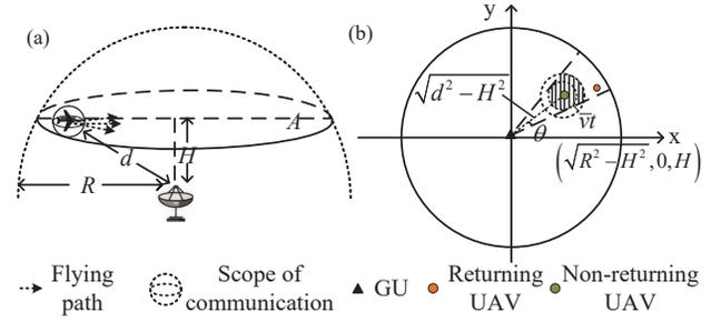
Fig. 6: UAVs' 2-D space of activities. (a) the scene diagram of the UAV's activity range in 2-D. (b) the top-view geometric diagram of the UAV's activity range in 2-D.
