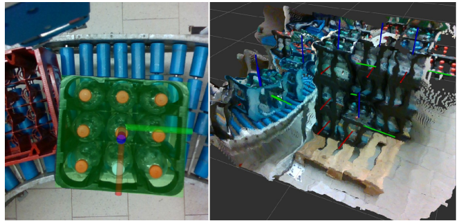
Fig. 10: Detection of beverage crates (Intel® RealSense D435)
