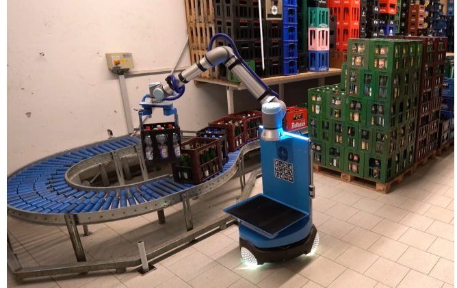
Fig. 1: Beverage logistics with a mobile handling robot
