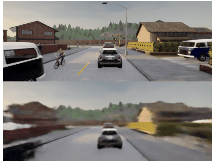
Fig. 1. The bottom row shows a scene reconstruction of a world model [6]. Compared to the ground truth, the model cannot recover all scene components, such as the bicyclist. This phenomenon can be exploited through a clear definition of normality and targeted training to detect anomalies.
